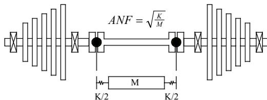
Because most dry couplings exhibit either nonlinear axial spring rates or are well damped, large axial deflections are not found at or near ANF's. In fact, there has never been a documented case of a coupling failure contributed to ANF. Therefore, the third edition of API 671 has virtually eliminated this previous requirement. Only undamped flex element couplings with linear spring rates are required to avoid having calculated ANF's within 10% of the operating speed range.
