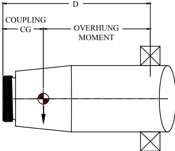
The way in which the coupling's effective CG is calculated is to assume that negligible moment from the coupling weight can be transmitted across the flex point - thereby treating the coupling's flex point (disc pack, flexible diaphragm, or gear mesh) as a pin joint. The closer the flex point is to the equipment bearing, the less the resulting moment from coupling weight causing the shaft to deflect.
