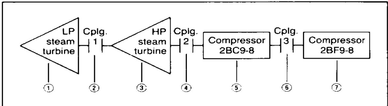
We will be looking at coupling #2 (position 4). The combined horsepower requirements for coupling #2 was 27,500 HP speed 10,300-11,000 RPM. The Figure 2 below shows the original gear coupling.
